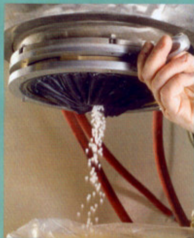
Blended compounds are discharged at a controlled rate through the mixer's iris valve.
