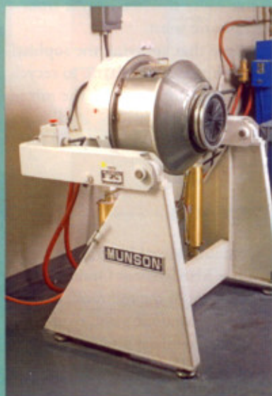
Munson MX-1-SSJ miniature rotary batch mixer with mixing vessel jacket plumbed to a water-heating unit.
