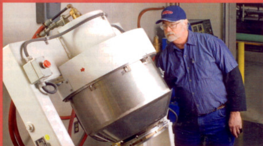
A General Cable technician tilts the mixer to vertical for discharging.
